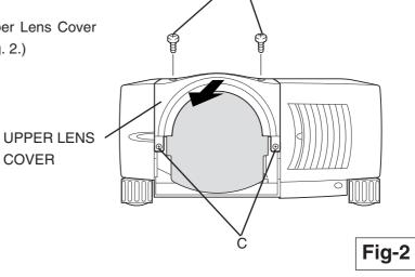
Remove 2 Screws D and Cover Plate from the back of the Upper Lens Cover. (See Fig. 3.)
